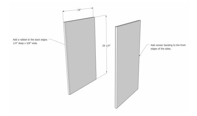
If using a 1/4" plywood backing for the cabinet, add a 1/4" deep x 3/8" wide rabbet to the back edge of the side pieces of the cabinet using either a rabbeting bit on a router or a dado stack on a table saw.
