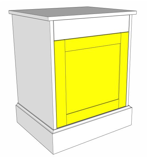
Using inset hinges (i.e. frameless inset hinges or euro style hinges), install the cabinet door. Use equally stacked playing cards to achieve an even 1/8 gap around the door. Install the door hardware and a magnetic stop on the opposite side of the cabinet.
