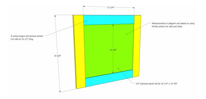
**If using pocket joinery**, cut the rails and stiles based on the diagram above. Drill 3/4" pocket holes into the rails. Add a 1/4" wide x 3/8" deep groove to the inside edge of the rails and stiles to fit the 1/4" plywood panel. Set the plywood into the grooves. Glue and clamp the rails and stiles together, then attach with 3/4" pocket screws.
