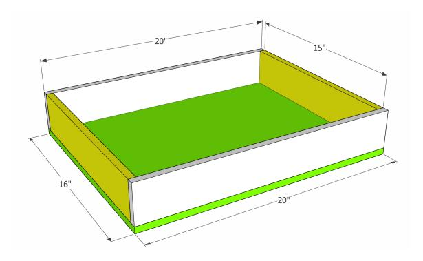
Drill 1/2" pocket holes into the 15" sides of the drawer box. Glue the ends and attach to the drawer front and back pieces with 1" pocket screws. Cut the bottom to size, glue and attach with 1" brad nails. Install the drawer into the cabinet using desired drawer slides (i.e. bottom mount or side mount).
