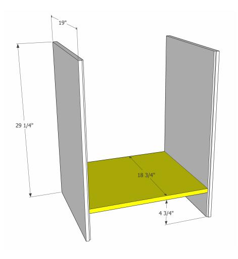
Before assembling the carcass of the cabinet, drill 3/4" pocket holes into the top, inside ends of the cabinet sides as well as 3/4" pocket holes into the two shorter ends of the cabinet bottom. Measure and mark 4 3/4" up from the bottom of the cabinet sides. Add glue to the ends of the bottom piece and set in place along the marks. Clamp and attach to the sides using 1 1/4" pocket screws.
