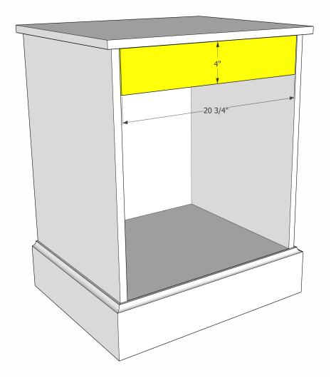
To install the drawer front, pre-drill the holes for the drawer pull hardware into the drawer front. Set the drawer front against the drawer box with an 1/8" gap around the top and sides. Stacked playing cards are a great way to set this gap.
