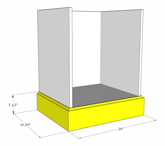
Measure and install the moulding to the base of the cabinet. The moulding can be made using a cove bit on a router, or left as a solid 1x6. Glue and nail the moulding in place with  $1 \frac{1}{4}$  brad nails. Fill the nail holes with wood filler, let dry, then sand with 220 grit sandpaper.
