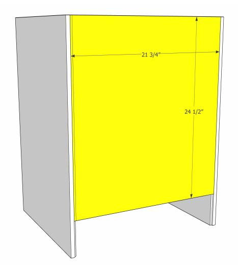
Add a bead of glue to the rabbeted grooves on the back of the cabinet carcass. Place the 1/4" plywood backing in the grooves and nail in place with 3/4" brad nails.
