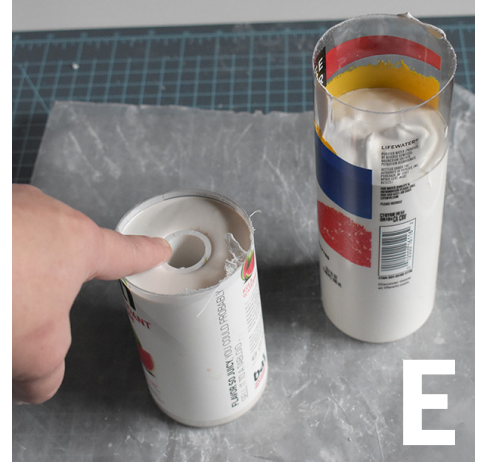
Push it down flush with the plaster
